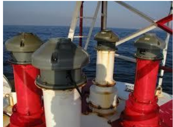
Wave Power Generator installed at a Large Buoy
