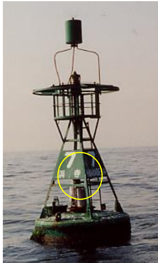
Lighted Buoy equipped with the Wave Power Generator
