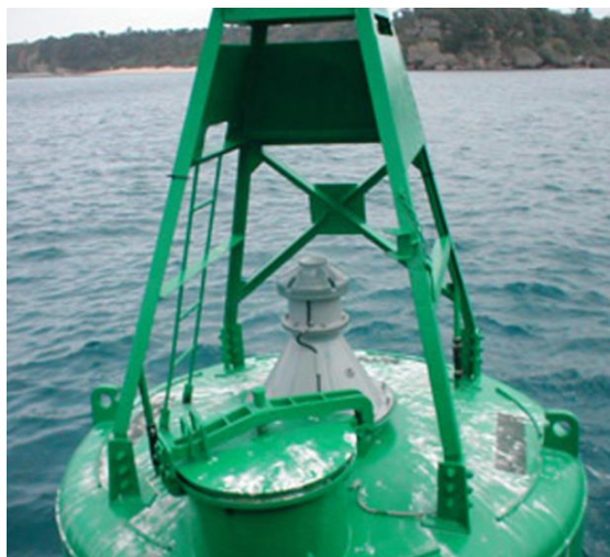
Lighted Buoy mounted Wave Power Generator
