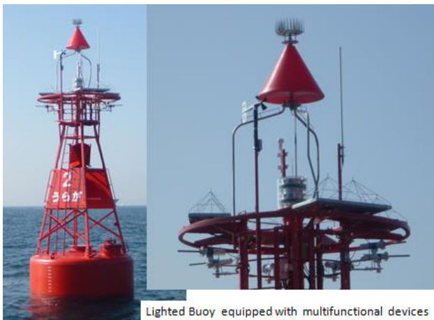
Lighted Buoy equipped with multifunctional devices
